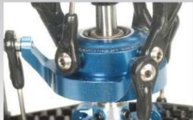
SWASH CONTROL: The swash is controlled by a 120° CCPM configuration with direct input linkages.
