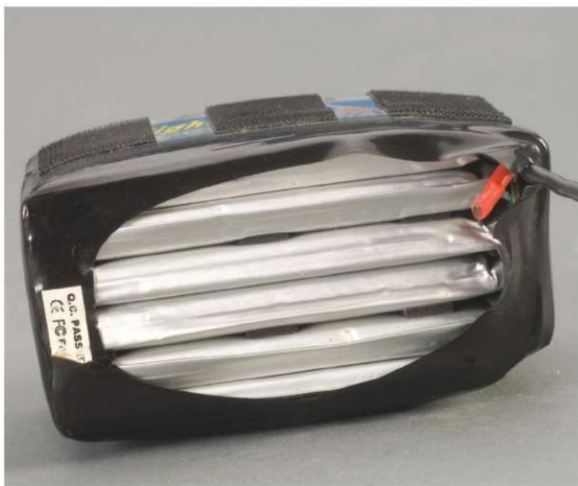
This is an example of a battery that is either being run too long each flight, or being pushed harder than its rated for. A puffed battery like this is at the end of its life cycle and is ready for disposal.
